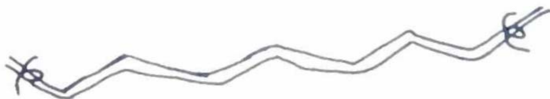
STRIP PULLED AND TIED EACH END.
