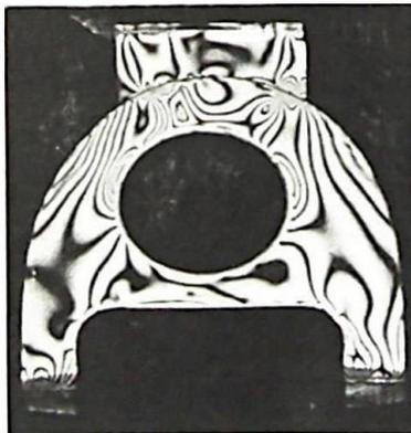
Fig. 2: Fringe patterns in photoelastic Model *CE*
