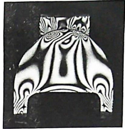
Fig. 3: Fringe patterns in photoelastic Model *BE*
